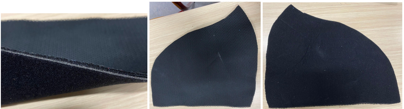
Figure 13 : Material chosen for Noé's comfort (top of the material : in touch with Noé's skin, bottom of the material : attach with velcro to the system)
