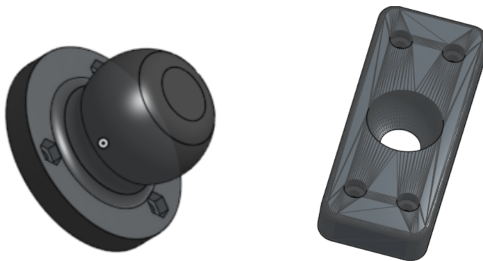
Figure 7 : CAO of the ball joint coupling's components. Left : Soft ball Right: Solid socket
