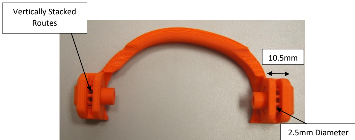
Figure 13-51: Vertically Aligned Holes Wrist Joint
