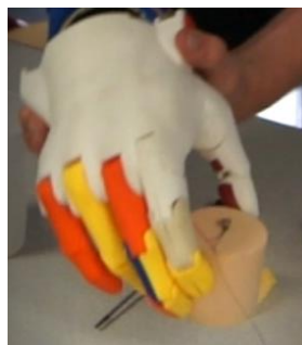
Figure 18-1: 50mm foam cylinder picked up by prosthesis.
