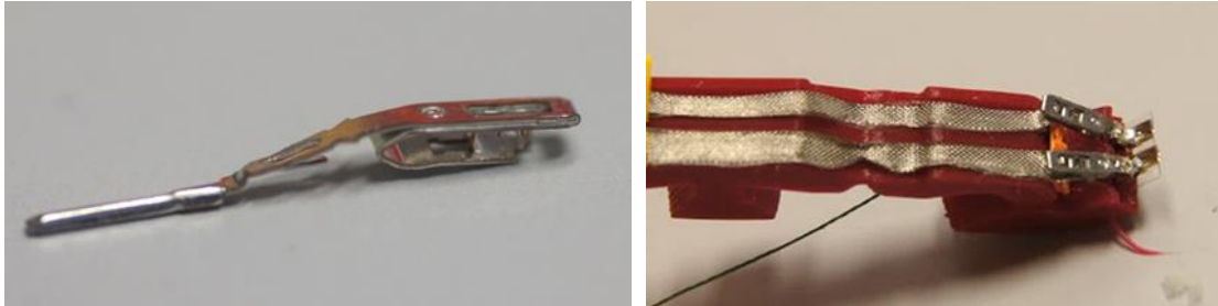
Figure 13-26: metal connectors connected to conductive fabric
