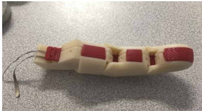
Figure 13-22: conductive fabric successfully routed through finger
