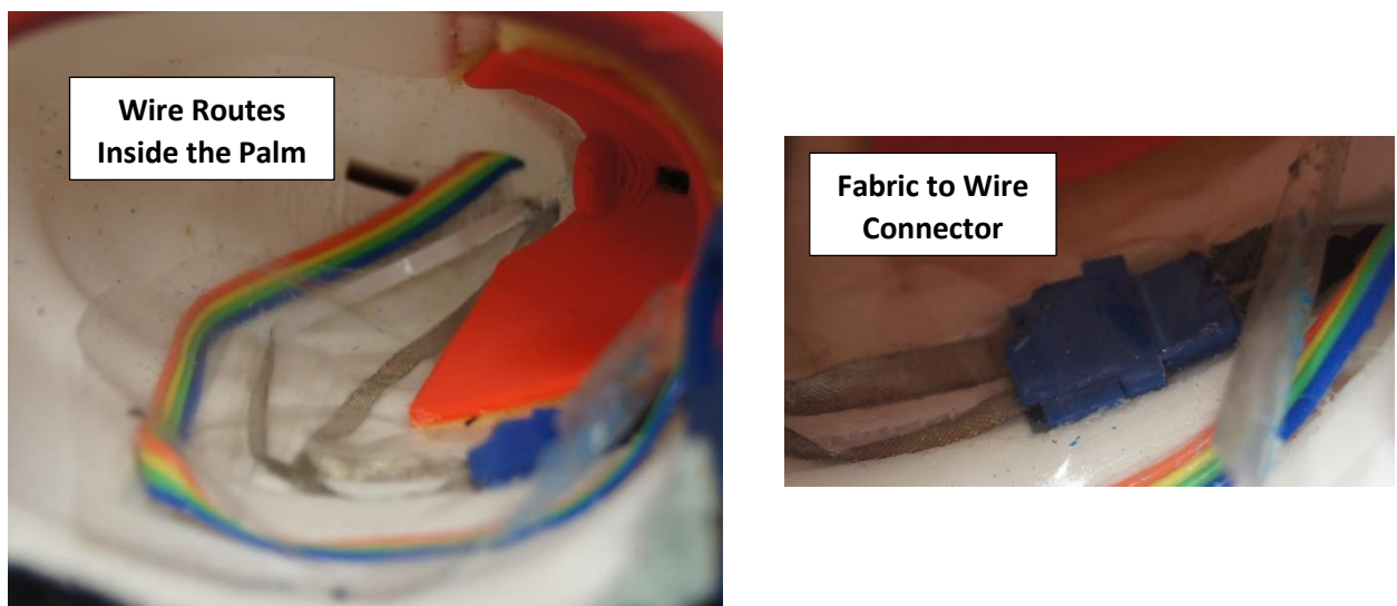
Figure 16-3: Wire Route in Palm Cavity with Conductive Fabric Connector
